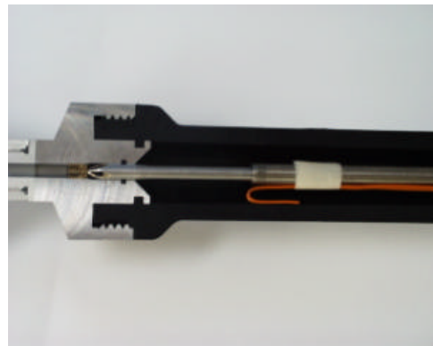
Fill stem & igniter wire inside a J motor
